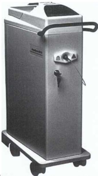
FIG. 7-28 Example of laser use. A, Nd:YAG laser unit with a power supply, control panel, fiber-optic wave guide, and probe. B, Laser probe and beam emanating from probe tip. C, Lased area on dentin (from Nd:YAG operated at 1.06 \mu\text{m} wavelength, 167 mJ/pulse, and 207 J/cm 2 power) showing physical modification produced by a single pulse. The hydroxyapatite crystals on the surface were melted and recrystallized with partial closure of the tubules. Surface roughness from tooth preparation was eliminated by the lasing. The area immediately adjacent to the lased site seemed to be unaffected. (A, Courtesy of American Dental Technologies, Inc., 5555 Bear Lane, Corpus Christi, Tex.; B, Courtesy of Dr. Art Vassiliadis, Sunrise Technologies, Fremont, Calif.; C, Courtesy of Dr. Joel White, Department of Restorative Dentistry, UCSF School of Dentistry, San Francisco, Calif.)
