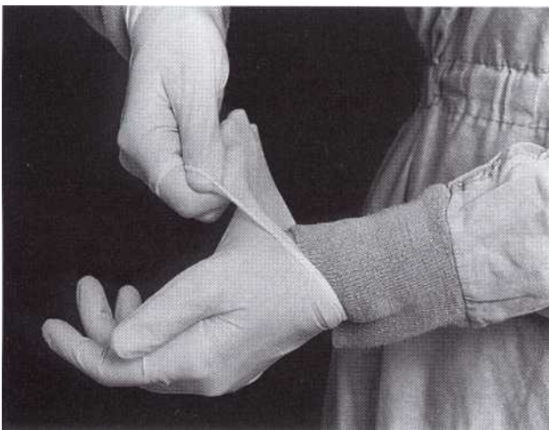
FIG. 8-5 To remove a contaminated glove, pinch the palm side of the outer cuff surface with the gloved fingers of the other hand. Pull off the glove, inverting it. Both gloves can be removed simultaneously in this manner. Alternately, after removing one, insert bare fingers under the cuff to grasp and pull off the remaining glove. Discard gloves safely.
