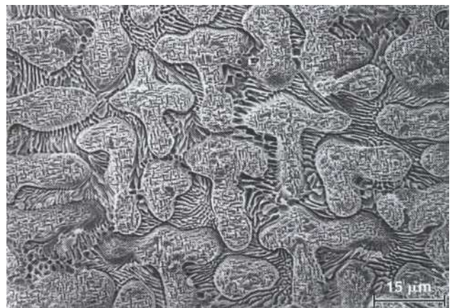
FIG . 5-29 Scanning electron micrograph of Rexillum III (Jeneric/Pentron, Wallingford, Connecticut) after electrochemical etching with 0.5N nitric acid for 5 minutes. (Special thanks to Dr. Glen Imamura for preparing this specimen.)
