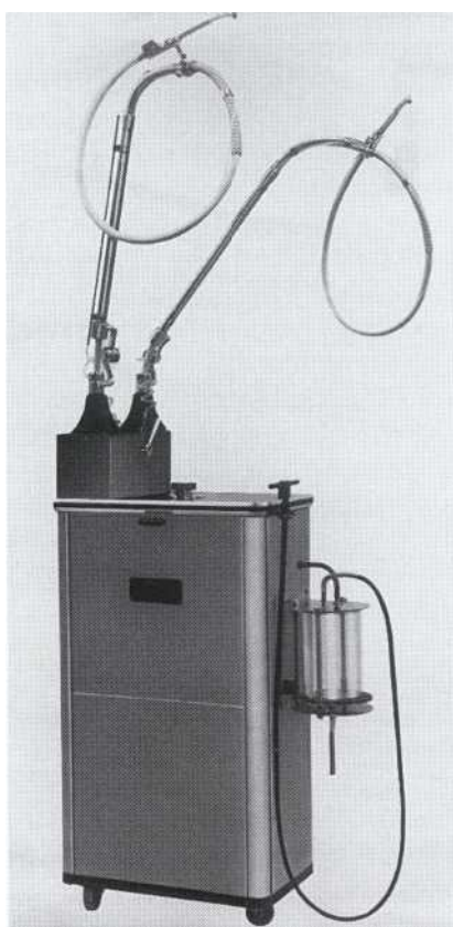
FIG. 7-25 Turbo-Jet portable unit (circa 1955). A small turbine in the head of the angle handpiece is driven by water circulated by a pump housed in the mobile base.
