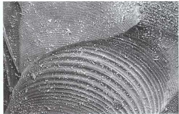
FIG 2-28 Smear layer on cut dentin preparation surface. Swirls on surface are from end of a carbide bur. (From Marshall GW, Marshall SJ, Bayne SC: Restorative dental materials: scanning electron microscopy and x-ray microanalysis , Scanning Microsc 2(4):2007-2028, 1988.)
