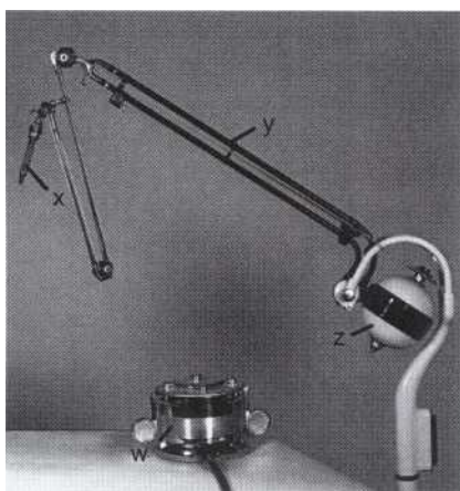
FIG 7-23 Typical equipment when an electric motor is used as source of power: foot control with rheostat (w), belt-driven straight handpiece (x), three-piece adjustable extension arm (y), and electric motor (z).
