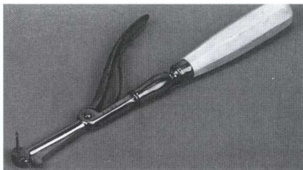
FIG 7-21 Early angle hand drill for indirect access preparations (circa 1850). The bur is activated by squeezing the spring-loaded handle.
