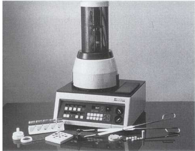
FIG. 14-15 Device for pressing heated ceramic. (Courtesy of Ivoclar, North America.)
