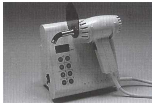
FIG 4-71 Example of visible light-curing unit for use with composites, bonding agents, and other light-curing materials. The main power supply is connected to a pistol-grip light gun that generates a beam that is passed through the fiber-optic tube. A shield is supplied to protect against direct observation of high-intensity light at the tip (Courtesy Kerr-Sybron, Orange, Calif).
