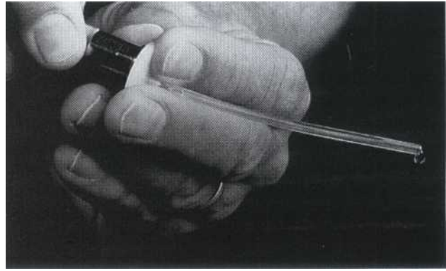
FIG. 8-19 This device is used to detect retraction of water supplied to the high-speed handpiece by older units when the foot control is released. If water moves back into the plastic tube, a new check valve is needed in the handpiece waterline to prevent retraction of oral fluids during treatments. (Courtesy of A-DEC, Inc. Newberg, Ore.)
