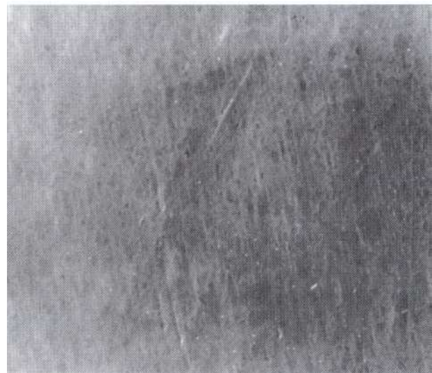
FIG. 11-9 Scanning electron micrograph of polished surface of a microfill composite (x300).
