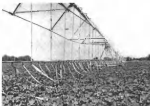
29-rasm. G'o'zani egatlab sug'orishda «Kuban» yomg'irlatib sug'orish mashinasidan foydalanish.
